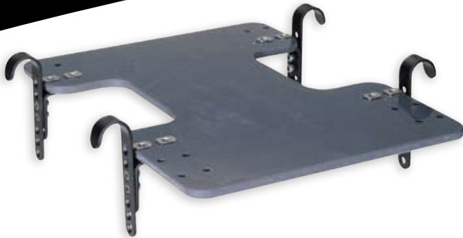
*VARILITE* Drop Base is made from durable and lightweight 3/8-inch (1 cm) PVC. Our L-J brackets are hardened steel for superior strength and durability. The hardware allows 4 inches (10 cm) of height adjustment and 15 degrees of angle adjustment—great for changing the seat-to-floor height or seat-to-back angle.
